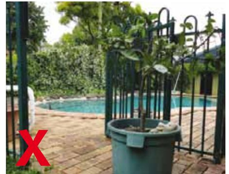
This gate is being held open by a pot plant, which could also be used to climb into the pool area, and must be removed.
